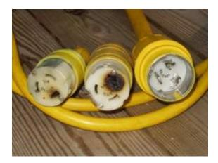
Feel the shore power cable. If it is hotter near the connector than it is in the middle of the cable, something is wrong.
